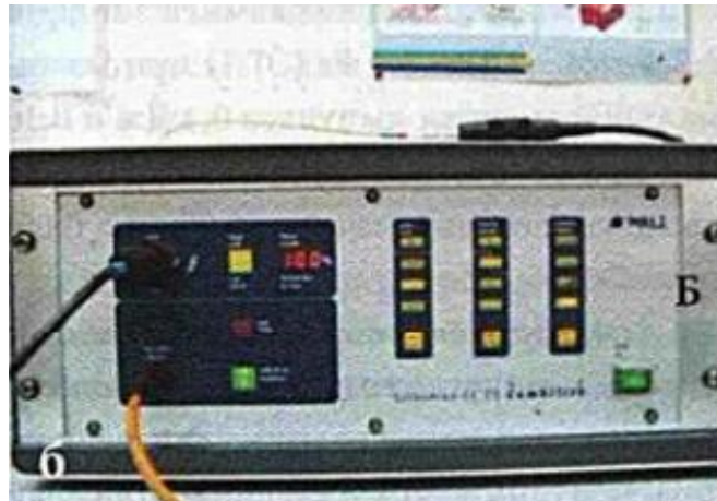
Fig.6. Instruments used in experiments. A. nanosecond electropulse lithotripter "Urolit-105M"; b. electrohydraulic lithotripter « Lithotron EL 25".
