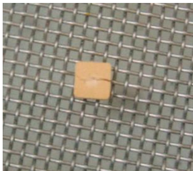
Fig. 4 a, b. Stages of destruction of an artificial "urinary stone" sample during the operation of a nanosecond electric pulse lithotripter (explanations in the text).
