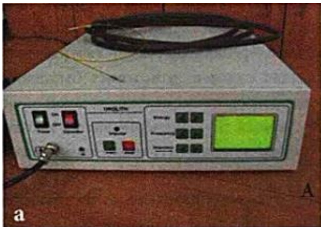
Fig.6. Instruments used in experiments. A. nanosecond electropulse lithotripter "Urolit-105M"; b. electrohydraulic lithotripter « Lithotron EL 25".
